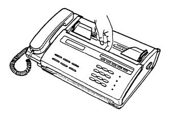
2. Disassemble the white roller. Both ends of the roller are terminated with bushings which are snapped shut with small tabs. Push the tabs slightly inwards in the direction of 'A', then rotate in the direction of 'B' until it reaches the slot as shown in the figure below. Then pull the roller upwards in the direction 'C'.
